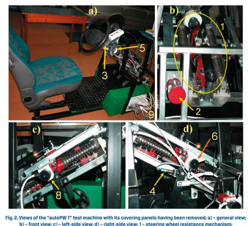
Fig. 2. Views of the "autoPW T" test machine with its covering panels having been removed; a) – general view;
