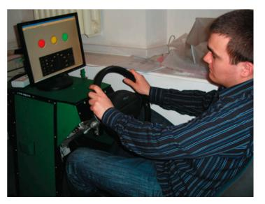
Fig. 1. General view of the "autoPW T" test machine during a driver examination
