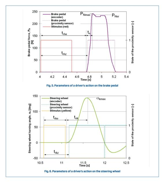
Determining of driver reaction time on the "autoPW-T" test machine
